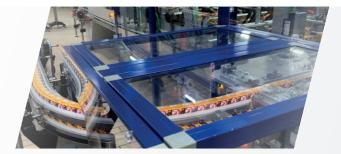
**FAST FEED:** 90° infeed system. It avoids the use of lane divider and metering section at packer infeed. It improves hygienic design, simplifies change overs and improves flexibility in line layout design and machine compactness. It can be integrated with 90° and 180° package rotation device for facing or cap orientation inside the pack collations.
